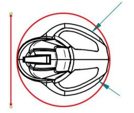
Cross-Country ski poles with Cross-Country skiing tips must be used. Alternatively poles tips must have safety rigid plastic protections with diameter ≥30 mm. These protections must be placed maximum 45 mm above the metallic tips.
